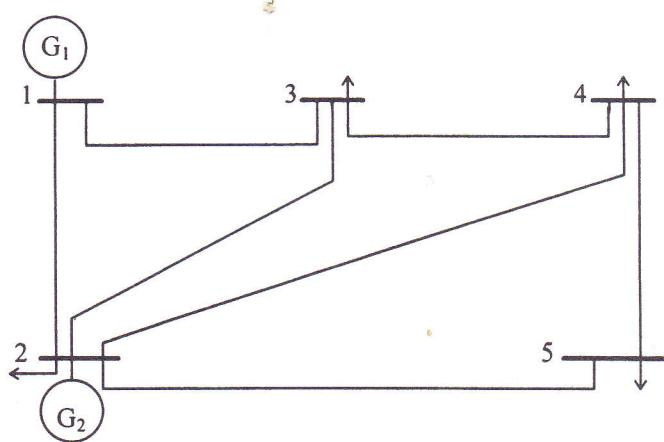
Fig. 2. One line diagram of the sample system.
